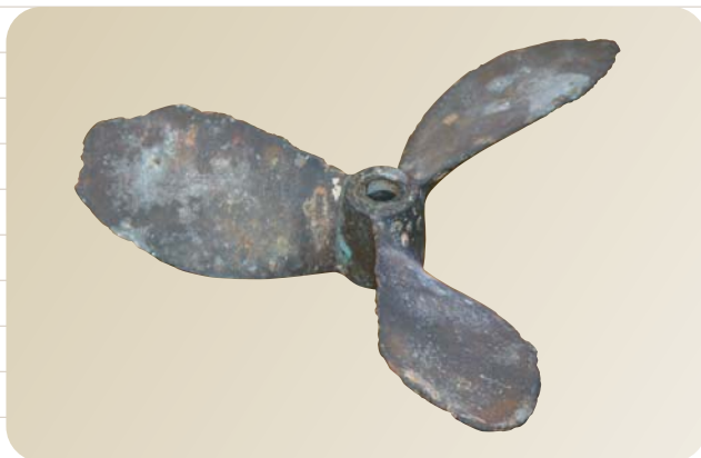
▲ A propeller taken from a ship when Dokai Bay was at its dirtiest. It took a relatively short amount of time for the propeller to become this corroded.
